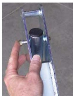
**Step 2:** Start 1/2"-22 self locking nut on to bolt. Tighten bolt using two 3/4" wrenches.
