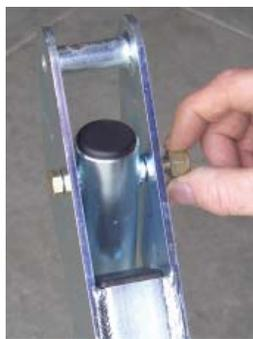
**Step 3:** Swing link arms up to handle. Insert the long 3/8"-24 bolt through link arms and handle. Install flat washer on bolt. Start 3/8"-24 locking nut on bolt.
