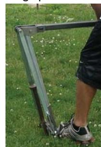
**Handle Extension:** Remove clevis pin in handle, extend inner handle to desired length and replace clevis pin. See below.
