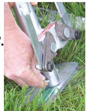
**VERY IMPORTANT:** If you are pulling a stake from a stake bar or frame plate, put the metal base of the JackJaw unit **ON TOP** of the bar or plate. You must pull the stake straight out of the bar or plate. If the unit is on the ground next to the bar or plate, a slight misalignment can cause the stake to bind with the bar, making it difficult to pull from the bar.
